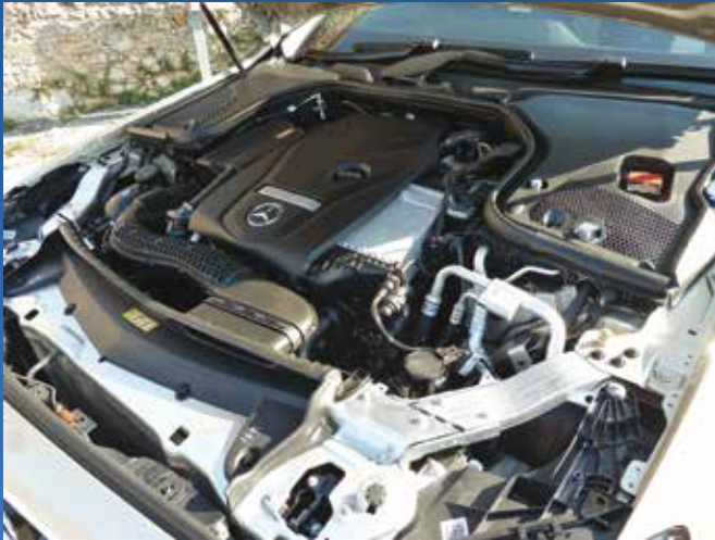
Under the bonnet more could be seen of the four-cylinder 245hp engine than on a lot of recent Mercedes. Bright metal alloy body parts were also prominent.
