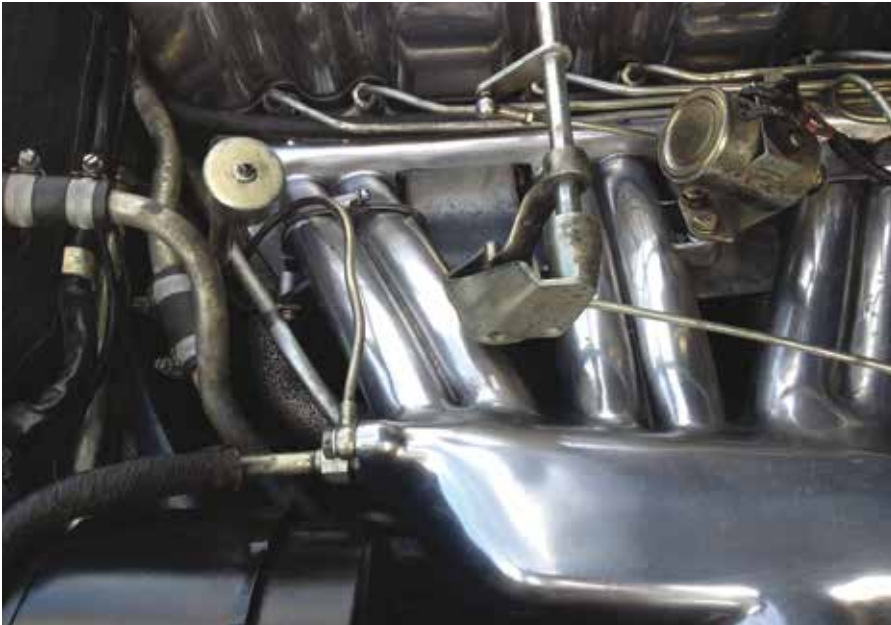
The small pipe from the gearbox can be seen coming up by the dipstick and terminating on the left end of the inlet manifold. As a temporary repair this pipe we disconnected from the inlet manifold. The manifold and open pipe end were both temporarily blocked.
